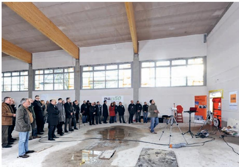
Blower door test: The necessity of tight seals became most obvious in critical areas like the points where the roof beams penetrate the walls. For demonstration purposes, a narrow joint was left unsealed, allowing strong draughts to be measured here.
