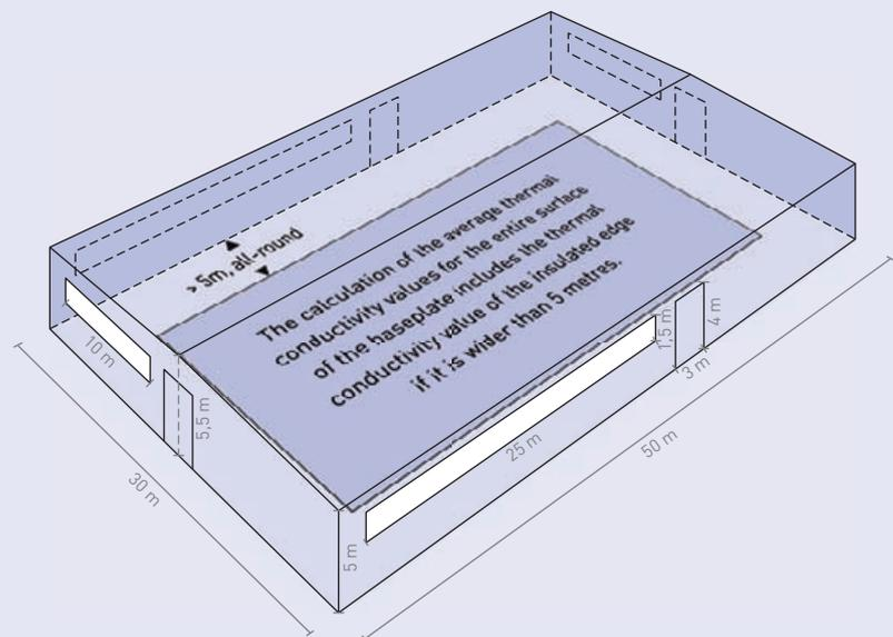
Average thermal conductivity value of the opaque construction elements:
