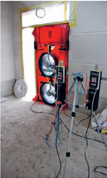
The better the insulation of a building, the more important its heat losses due to untight transitions of construction elements. The permanent air tightness of joints can be proven in a blower door test.
